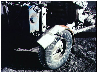
Apollo 17 Right Rear Fender Repair
